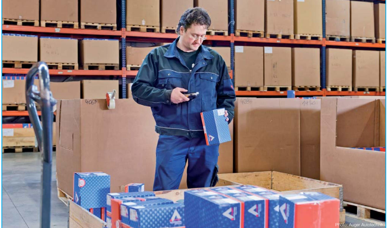
The barcode and GS1 DataMatrix, which are both integrated into the packaging label, are read with the 2D barcode scanner.
